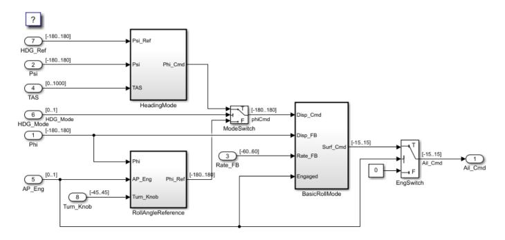
This model implements a basic roll axis autopilot algorithm, which controls the aileron position of an aircraft.
